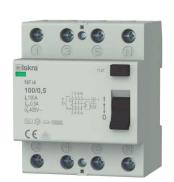
Type F - sensitive to residual currents as type a and in addition to residual currents with mixed frequencies
